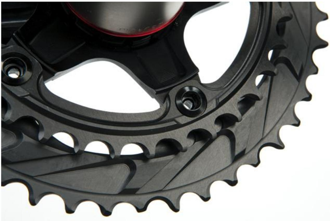
Every ramp on WickWerks chainrings is designed to lift the chain onto specifically designed teeth, which leads to ultra-smooth front shifting. Photo: VeloNews.com
